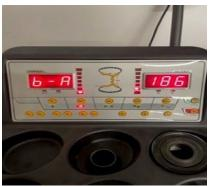
12. Pull Distance Gauge out and put to Flange – note distance on distance gauge. The number on the right must match the number noted on the distance gauge.
